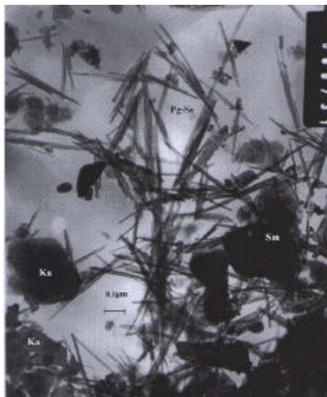
Fig.9. TEM of palygorskite-sepiolite fibers in a sediment-clay assemblage with kaolinite, smectite and other minerals in a sample at
